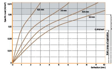
Diagram 2: Load deflection curve, using the example of Sylomer® SR110
